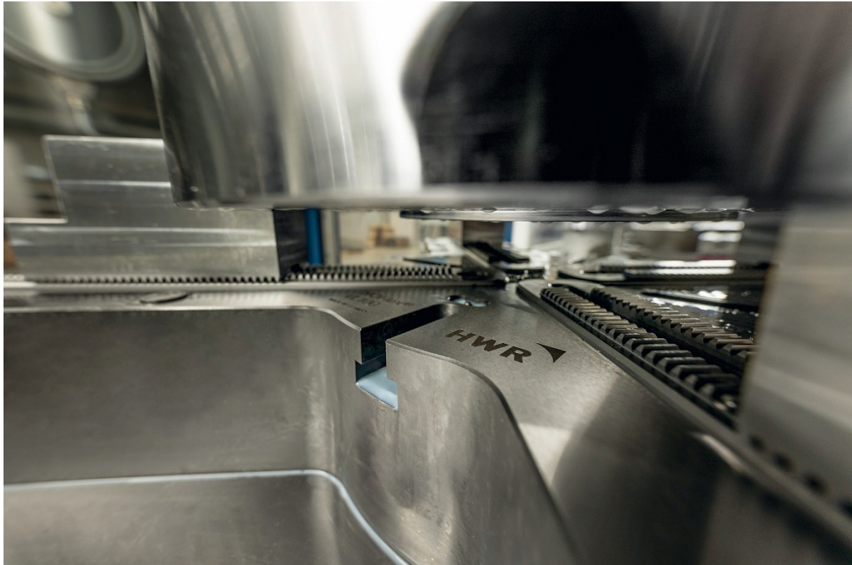
The clamping jaws are adjusted on the toothing of the "INOFlex VL 100" rotary chuck. Photo: HWR Spanntechnik / Mario Irmischer
